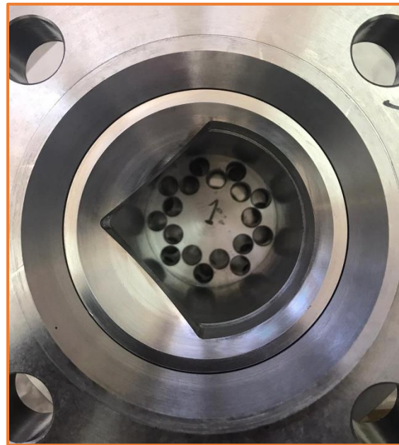
Segmented seat and a strainer installed inside the tail-pcs.
